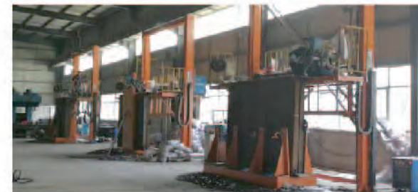
埋弧焊机 / Submerged arc welding machine 工作尺寸 / Working size 4000mm*4000mm
