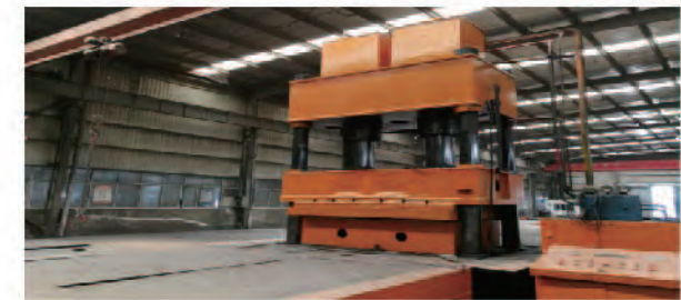
管板油压机 / Oil press machine 工作尺寸 / Working size \Phi 2300mm*100mm
