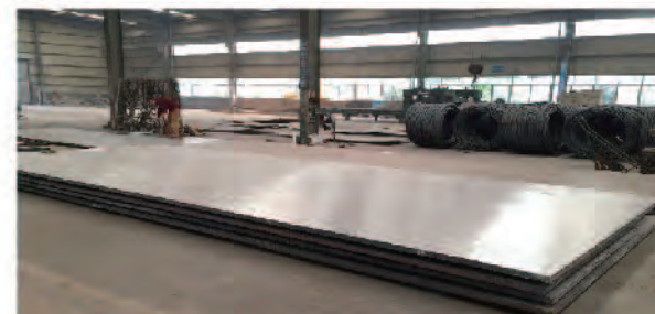
钛合金TA2 +Q345B复合板-北京龙源环保工程有限公司 Supplied Titanium TA2+Q345B Clad Plates to Longyuan Environmental for Power Plant
