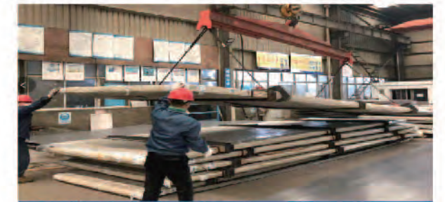
钛合金B265 Gr.2+A516 Gr.70复合板-BHEL/NTPC火力发电厂 Supplied Titanium B265 Gr.2+A516 Gr.70 Clad Plates to BHEL for NTPC Coal-fired Power Plant
