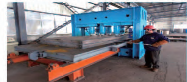
压力组对机 Package Assembly Machine (oil press) 工作尺寸 / Working size: 2600mm*4500mm
