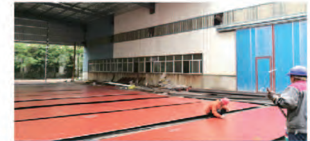
不锈钢SUS304+Q245R复合板-太阳造纸纸浆塔 Supplied Stainless Steel Clad Plates S31603+Q245R for Sun Paper, Paper & Pulp Tanks
