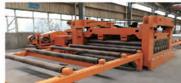
11辊矫直机 / 11-roll leveling machine 工作尺寸 / Working size: 2mm-14mm*2300mm*L
