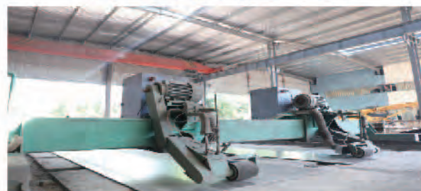
TIG自动拼焊平台 / Automated Welding Platform 工作尺寸 / Working size: 2mm-14mm*4000mm*12000mm
