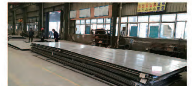
钛合金TA2 +Q235B复合板-北京清新能源/徐矿电厂烟囱改造 Supplied Titanium TA2 +Q235B Clad Plates to Beijing SPC for Power Plant
