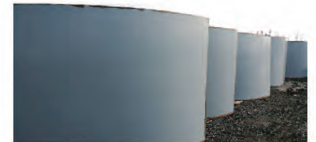
钛合金TA1 +Q235B复合板-中能建设电厂 Supplied Titanium B265 TA1 +Q235B Clad Plates for CEEC Power Plant Funnel Shell
