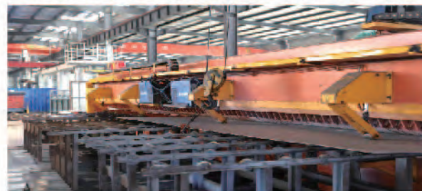
TIG自动拼焊平台 / Automated Welding Platform 工作尺寸 / Working size: 2mm-14mm*4000mm*12000mm
