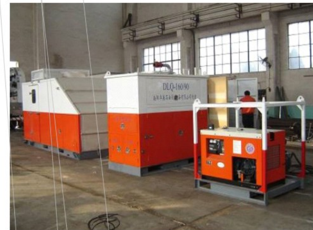
Separated skid-mounted logging unit
