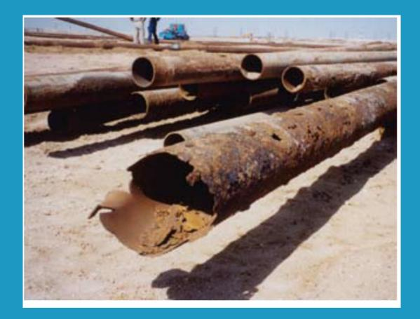
Carbon steel is suseptible to high levels of errosion and corrosion, C.S can also suffer from internal scale build up thereby reducing pipeline performance
