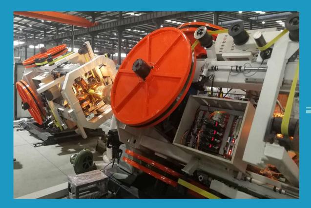
FPT use wrapping technology allowing for the productoion of both Metallic or Non-metalic reinforcement tapes
