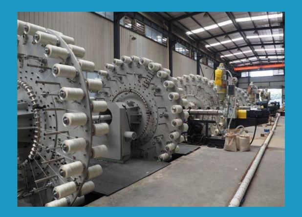
FPT use spiral winding equipment with bespoke design winders for higher pressure non-metallic reinforced pipe.
