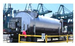
Envent designed its Portable Marine Vapor Control System to safely and efficiently destroy explosive vapors from marine cargo vessels during hydrocarbon loading activities. Our system complies with United States Coast Guard (USCG) regulations contained in 33CFR Parts 154 and 156 – Vapor Control Systems. Once on-site, Envent will work with our 3rd party certifying entity to acquire the United States Coast Guard (USCG) Certification Letter.
